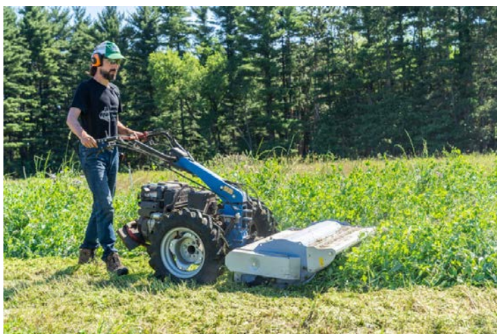
Flail mower on walk-behind tractor
